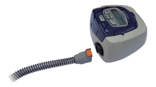
Step 2: Connect the adaptor to the heated tubing, and connect another end of the adaptor to the XD100 (Along the direction of the arrow mark of the adaptor);
