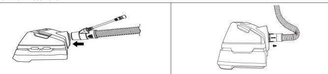
Step 3: Connect the machine-end cuff of the heated breathing tube to the air outlet of humidifier.
