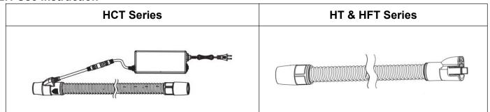
Step 1: Before installation, check the whole heated breathing tube unit for damage.
