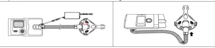
Step 4: Connect the user-end cuff of the heated breathing tube to the ventilation mask, nasal cannula, trachea cannula or other products.
